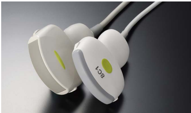
Figure 5 Conventional transducer (left) and thin-convex transducer, PVT-475BT (right) The contact surface of the thin-convex transducer is only 9 mm thick, half that of the conventional transducer.
